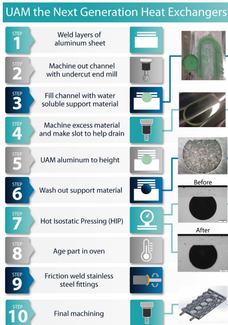
Figure 3 - Process steps for JPL test heat exchangers.
