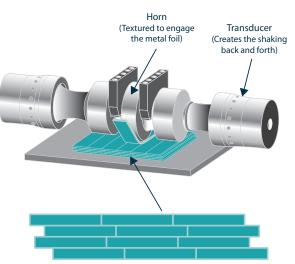
along the way and for part finishing. By combining a hybrid system, with both additive and subtractive processes, UAM can build complex internal geometries considered impossible to replicate with conventional manufacturing. For example, a metal heat exchanger can be made with aluminum and a layer of copper can be added to wick away heat.
