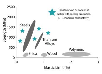
What if you could combine two, three, or even five metals in a graded laminate? One could then engineer a composite metal that meets the engineering needs.
