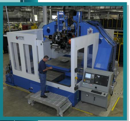
final dimensions at high accuracy. Full machine guarding is included (with a closed top). A water soluble coolant system comes standard with the machine and includes removable screen for chip removal. A secondary alcohol coolant system is also included for use during builds to keep the metal surfaces clean.
