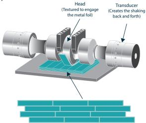
Hybrid metal additive is achieved by alternating Computer Numerical Control (CNC) machining interchangeably with foil layering to introduce precision smooth internal features during the printing process. Working in one machine as a hybrid system, with both additive and subtractive processes, UAM can build complex internal geometries considered impossible to replicate with conventional manufacturing.
