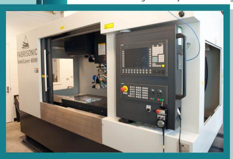
top). A water soluble coolant system comes standard with the machine and includes removable screen for chip removal. A secondary alcohol coolant system is also included for use during builds to keep the metal surfaces clean.
