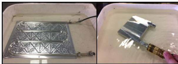
Figure 17: UAM Radiator and HX Subjected to Bubble Immersion Leak Testing
