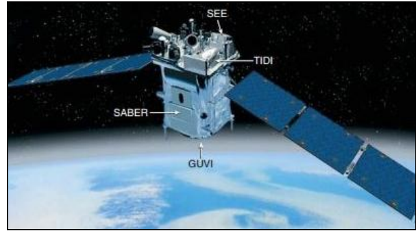
Figure 2: Original SABER Instrument on the TIMED Spacecraft 4
