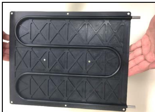
Figure 18: As built UAM Radiator Panel with Black Anodize Surface Treatment
